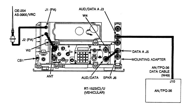
Figure 1. Cabling for AN/TPQ-36 to SINCGARS Radio Set
